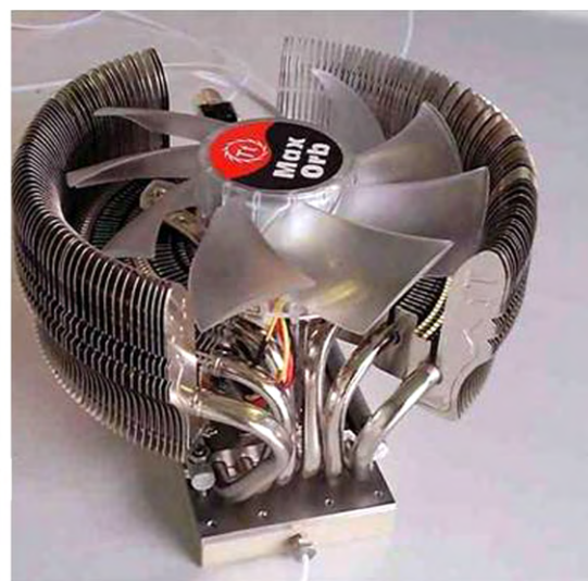
Fig. 9. Schematic of the microstructured reactor (left). Image of the mounted heat pipe on the reactor (right). The fan was not in use during the experiments.
