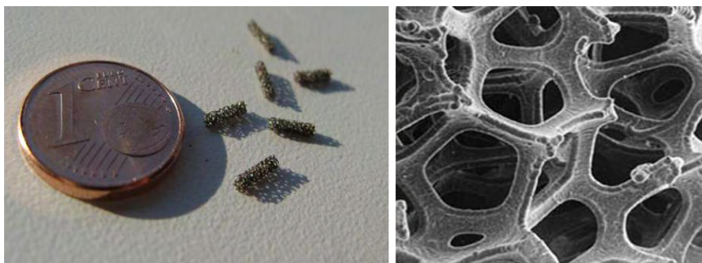
Fig. 4. Nickel foam (Recemat™) packing material with a diameter of about 2.1 mm (left) and SEM image (right).
